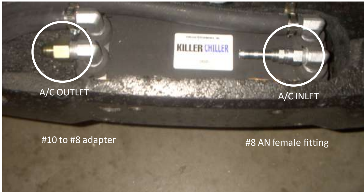
Figure 2. Detail of installed KC HE.
