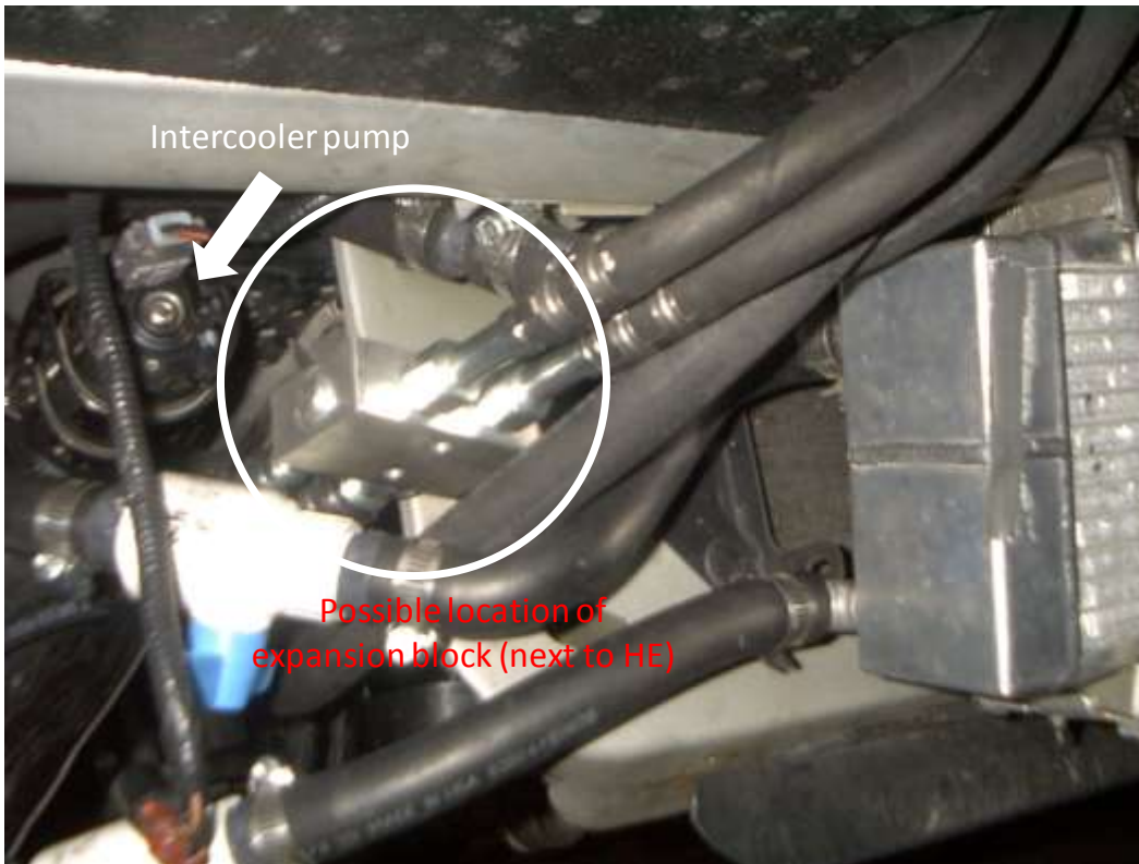
Figure 3. Detail of expansion block and #8 lines from KC HE.
